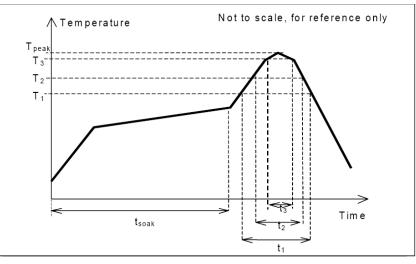
This profile is the minimum requirement for evaluating soldering heat resistance of components. Heat transfer method used for reflow soldering is hot air convection. The actual air temperatures used to achieve the specified profile is higher and largely dependent on the reflow equipment.
